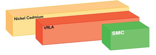
Typical volume of different battery types for 6 hours autonomy
