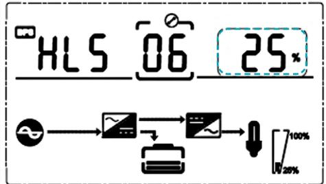
Pressing the DOWN button under the battery quantity setting or the UP button under the bypass voltage setting will take you to the bypass upper limit setting. You can select the upper bypass limit setting as follows:
