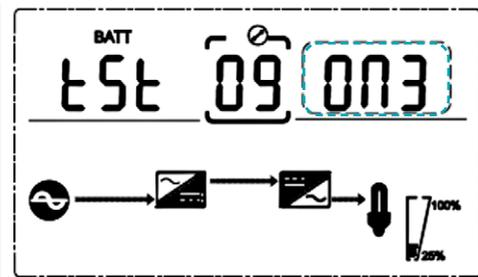
If you select ON3, the UPS can automatically switch to battery mode every 30 days. The battery self-test time is EOD (End Of Discharge).
