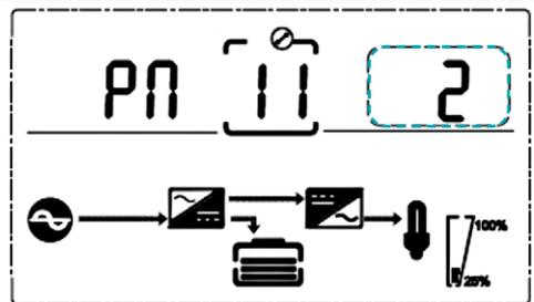
Press the DOWN key when setting the parallel ID or the UP key when setting the parallel redundancy quantity to move to the parallel quantity setting. You can set the parallel quantity as follows:
