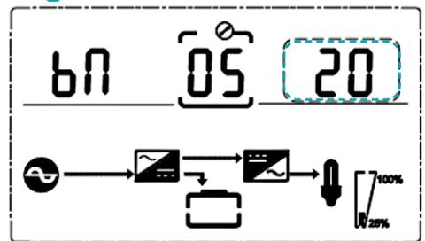
If you press the DOWN button under the battery capacity setting or the UP button under the bypass voltage cap setting, you will reach the battery quantity setting. You can select the battery quantity setting as follows:
