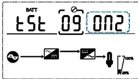
If you select ON2, the UPS can automatically switch to battery mode every 30 days. The battery self-test time is 10 minutes.
