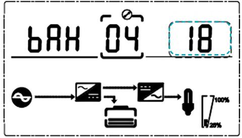
If you press the DOWN key under the frequency setting or the UP key under the battery quantity setting, you will reach the battery capacity setting. You can select the battery capacity setting as follows:
