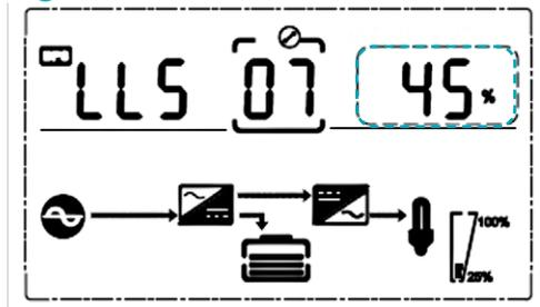
If you press down under the bypass voltage upper limit setting or if you press up under the buzzer mute setting, the bypass lower limit setting is activated. You can select the lower bypass limit setting as follows:
