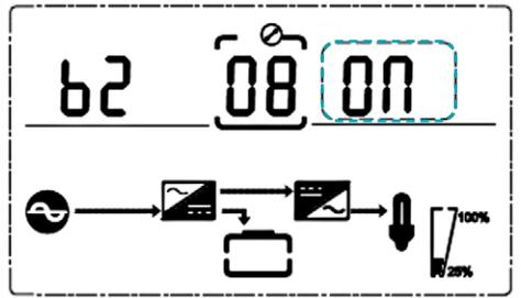
Press DOWN under the bypass voltage lower limit setting or press UP under the battery self-test setting to access the buzzer setting. Now the setting status flashes as shown in the figure.
