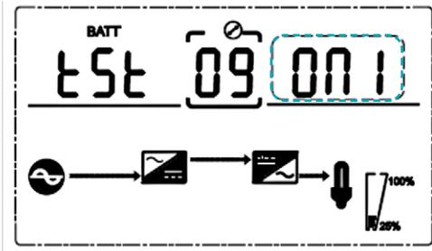
If you select ON1, the UPS can automatically switch to battery mode every 30 days. The battery self-test time is 10 seconds.
