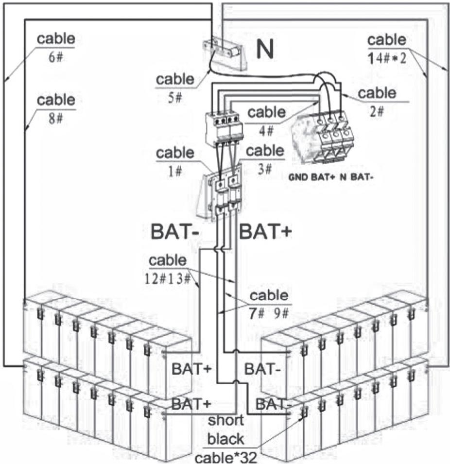
**Wiring diagram for the installation of 32 batteries**
