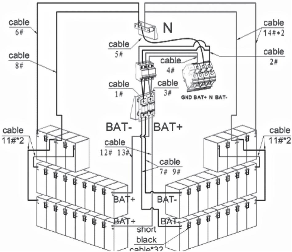
*Wiring diagram for the installation of 40 batteries*
