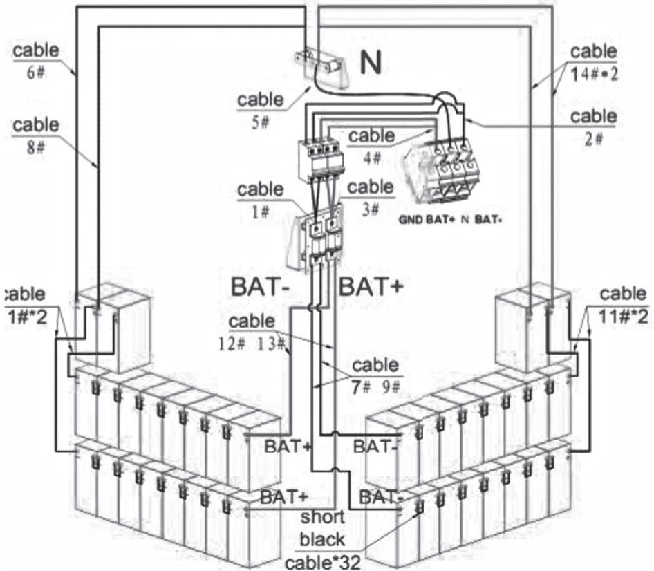
**Wiring diagram for the installation of 36 batteries**
